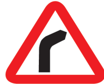
Right bend (Slow down. Keep left. Do not overtake, make a U-turn or park your vehicle)
