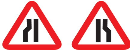
Road narrows on one side (Slow down. Do not overtake, make a U-turn or park your vehicle)
